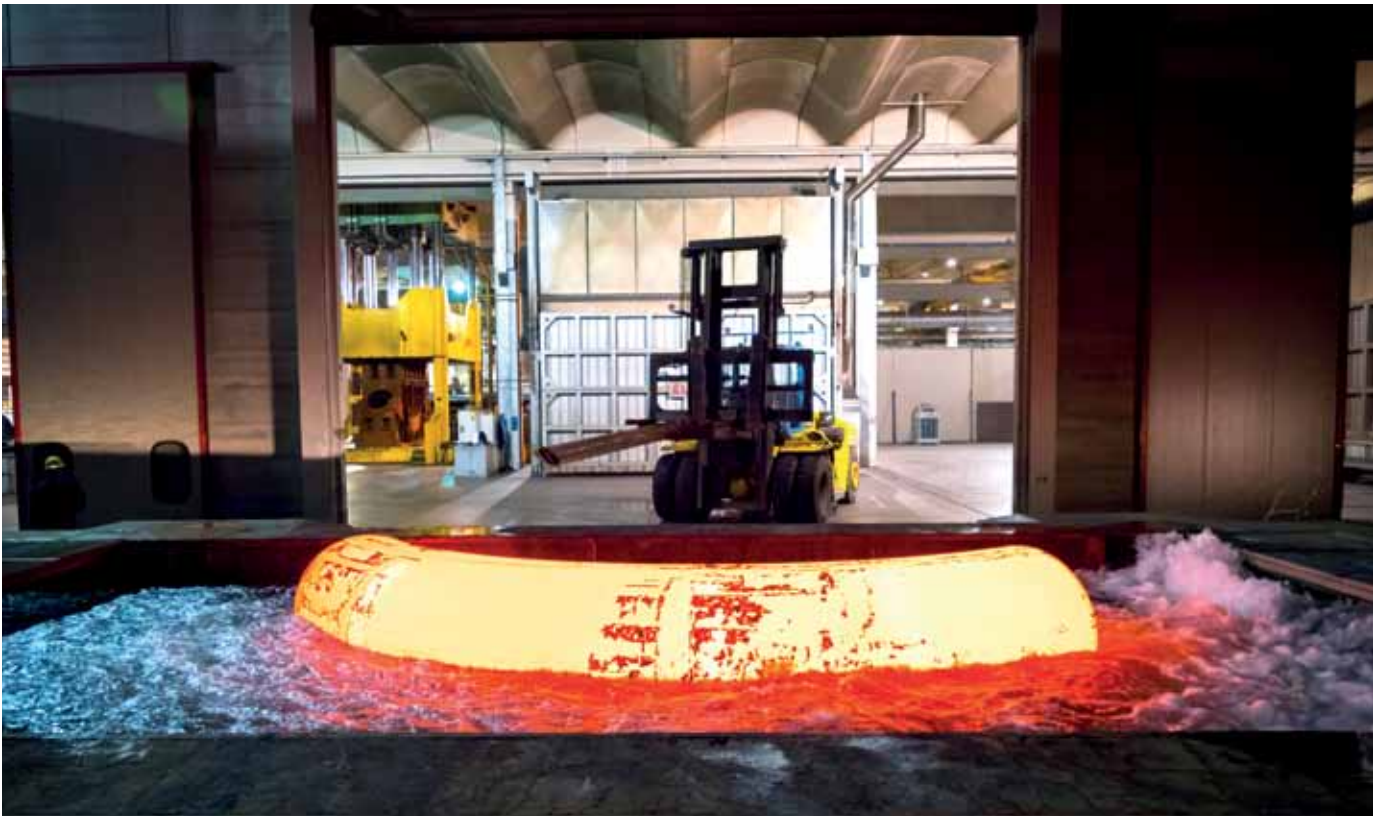
Above: some processing phases of large tee fittings Below: hot elbows in the large cooling tank during the heat treatment process
