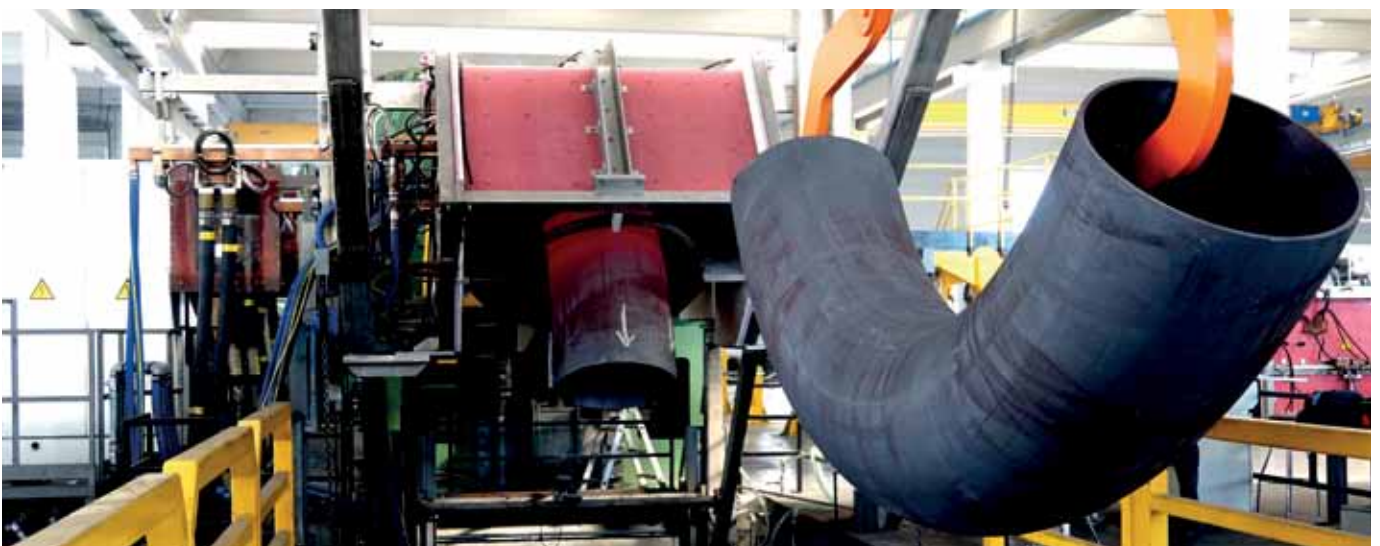
The large-dimension induction mandrel and bending machine MTC 1800 installed in the factory of Castel San Giovanni. Capable of unequalled production and a wide range of performances.
