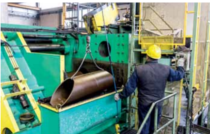
Above: the cold forming machine in the Podenzano plant for the production of tees up to 16" Below: the cold bending machine in the Calendasco plant for the production of elbows up to 16"
